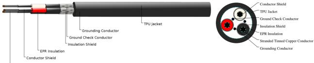
L Stranded Tinned Copper Conductor
